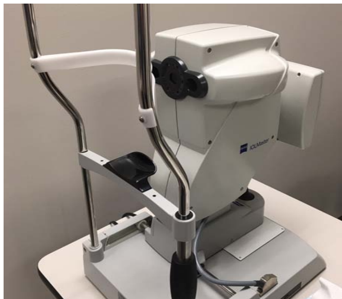
The IOL Master from Zeiss provides valuable axial length data, which is useful in guiding decision making in myopia management.
