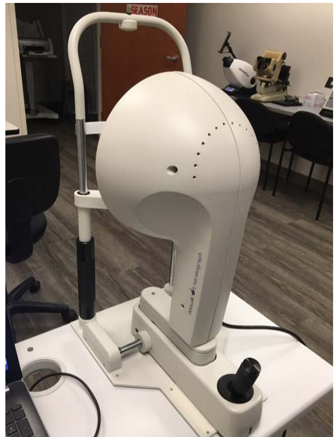
The Keratograph by Oculus is one of the many options for topographic measurement of the cornea. Topography is essential for monitoring patients undergoing orthokeratology treatment, and it provides valuable information for many conditions affecting the cornea.
